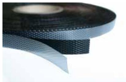
The resulting **BOC-9450 Edge Seal** is a multilayer construction consisting of a 35-mil adhesive layer of clear, aliphatic thermoplastic urethane (TPU) film bonded to a second, 15-mil layer of black, temperature-resistant aromatic polyurethane, and capped with an embossed polypropylene carrier sheet. The product is slit to the specific width of the laminated glass composite,
