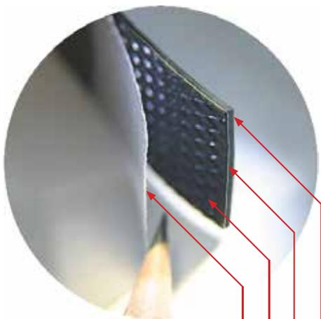
The clear, diamond-pattern-embossed carrier may be removed following lamination to the composite edge
