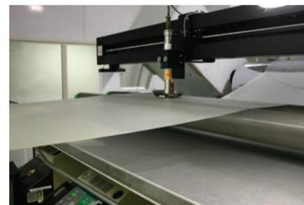
Digital in-line gauge measuring system for maintaining thickness control on SWM flat-die extruders.
