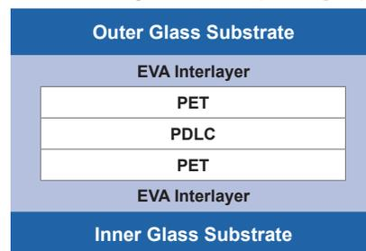
Fig. 1. Switchable glass laminate structure
